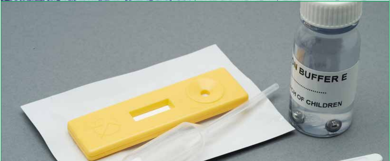
A Lateral Flow Device (LFD) kit as used for diagnosis of foulbrood in the field and in the laboratory
